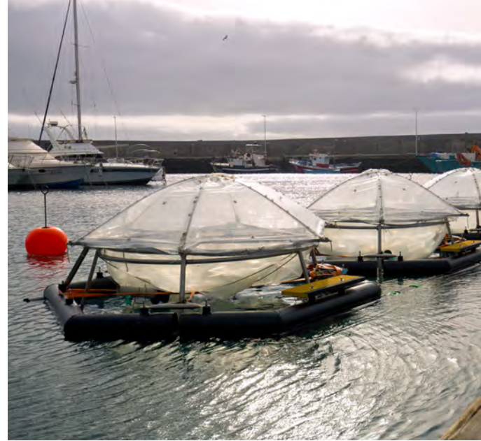
AN EXPERIMENTAL SETUP in the Canary Islands was used by Senior Research Scientist Steve Archer in 2021 to test the effectiveness of different ocean alkalinization treatments and investigate their impacts on marine life.
