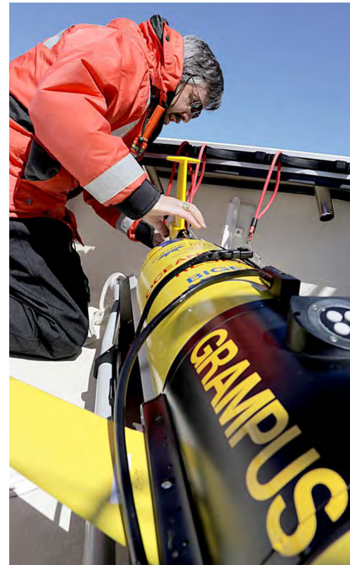
LEFT Senior Research Scientist Barney Balch attaches a tail to the autonomous glider "Grampus" before sending it on a three-week journey in the Gulf of Maine.
